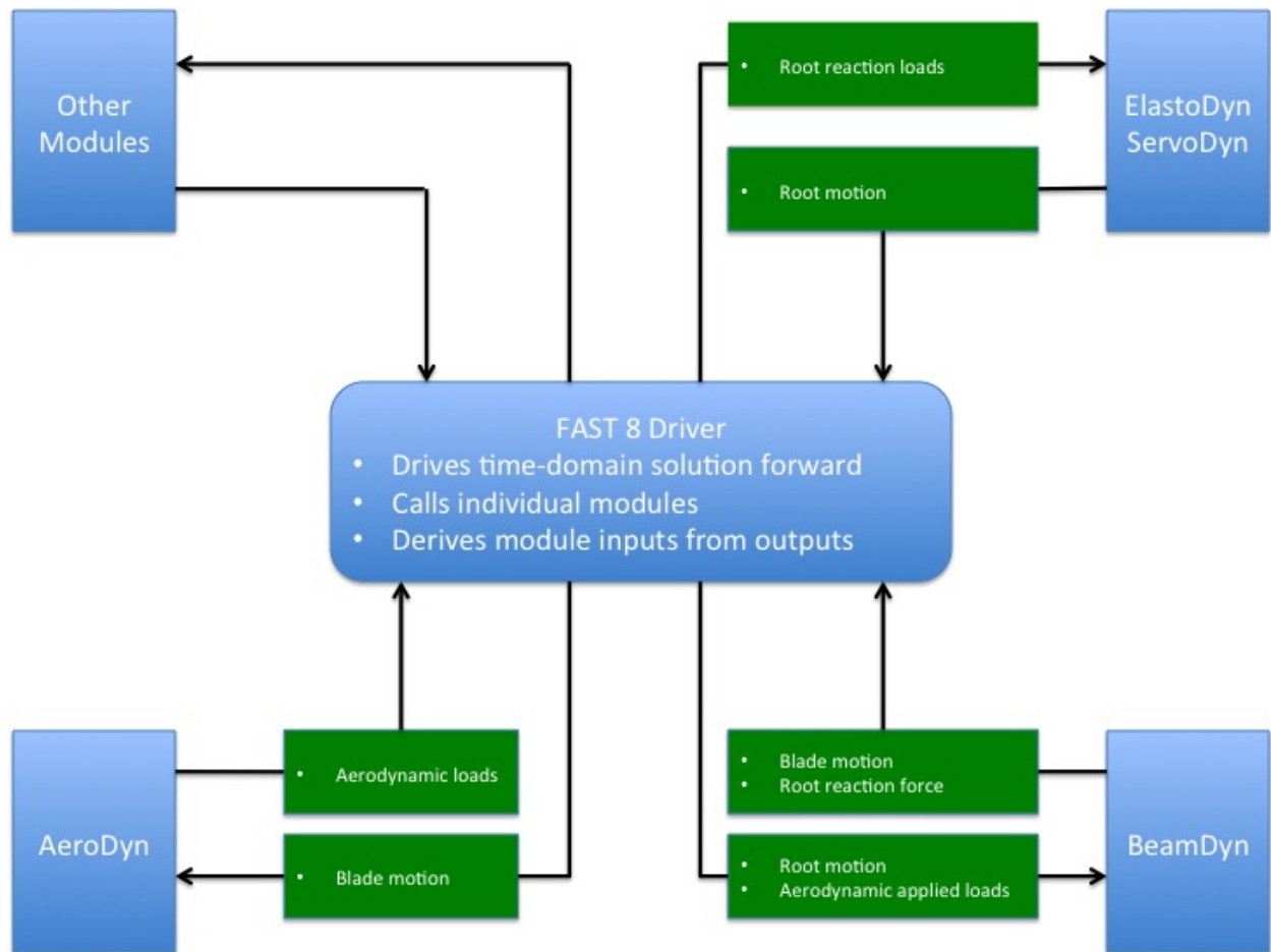
Figure 1. Coupled interaction between BeamDyn and FAST
