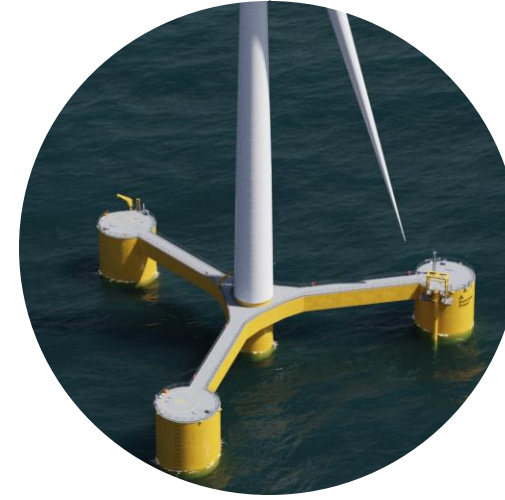
WindFloat TC Tubular, with center column, optimized for 15+ MW “Stiffer” Towers
