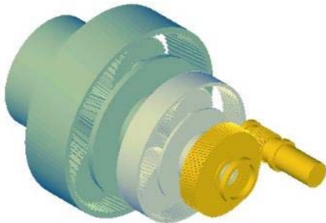
Baseline gearbox at 80 m/s tip speed
