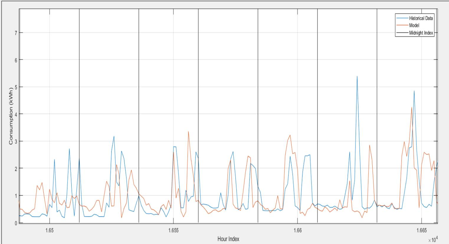
Using a state transition matrix based on the time of day and current energy use a Markov Chain Model was used to simulate a synthetic profile for a week.
