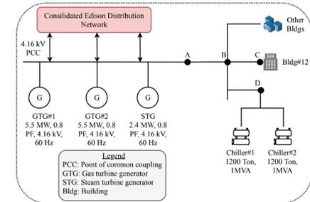
Figure 11. Schematic diagram of NYU microgrid depicting combined heat and power generation [95], where AB, BC, and BD are distribution lines modeled in the CC-OPF implementation.
