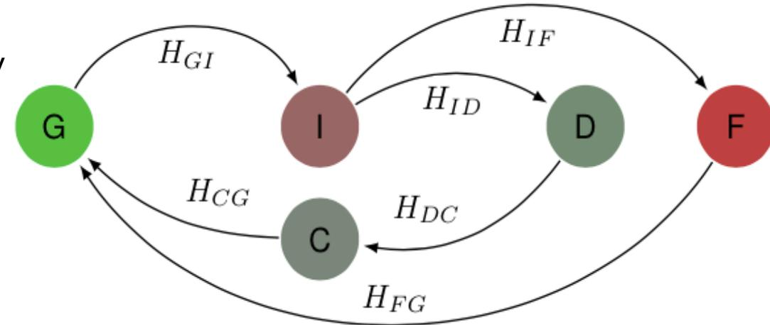
Fig: Semi-Markov Process (SMP) for cyberattacks on EVCSs.  $H(\cdot)$  defines the Cumulative Distribution Function (CDF) of the state transition time.
