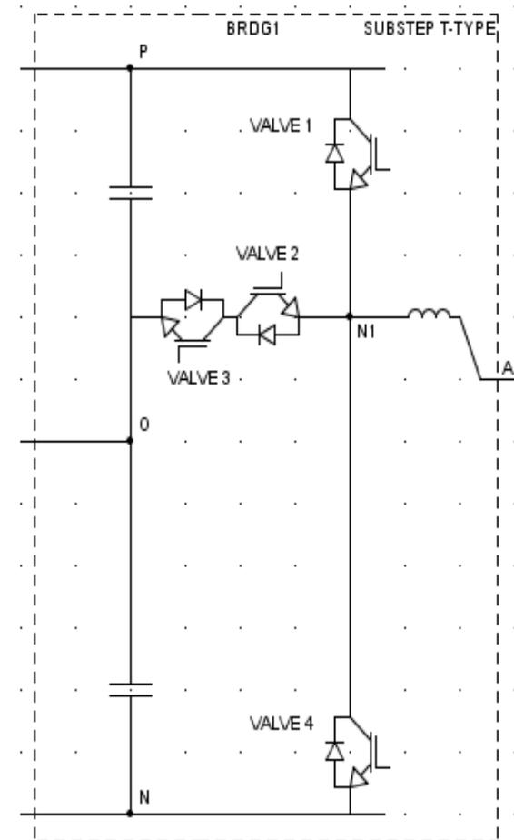
T-type resistive switching model
