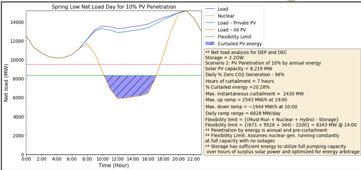
10% PV penetration is the lowest PV penetration scenario where curtailment occurs and the day pictured here has the highest curtailment at 20.28%.
