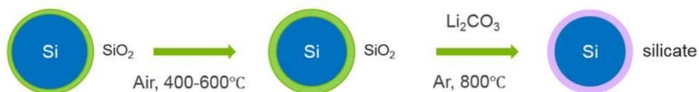
Figure 1. Diagram for the synthesis of  $\text{Li}_2\text{SiO}_3$ -coated silicon nanoparticles
