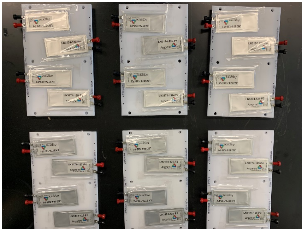
Figure 2. Single-layer pouch cells fabricated with 80 wt% Si electrodes versus NMC532 & HE5050 electrodes with “zintl phase” electrolytes (all pouch cells are not depicted in photo).
