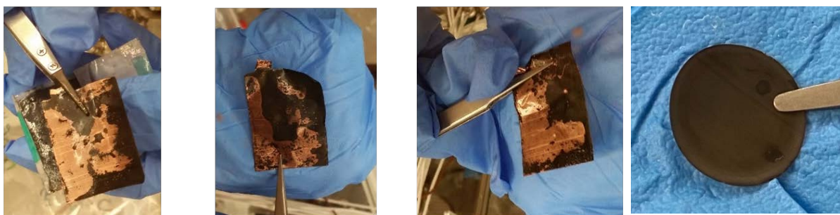
Figure 1. Selected SEM studies of three cycled pouch cell electrodes, and one cycled in a coin cell.
