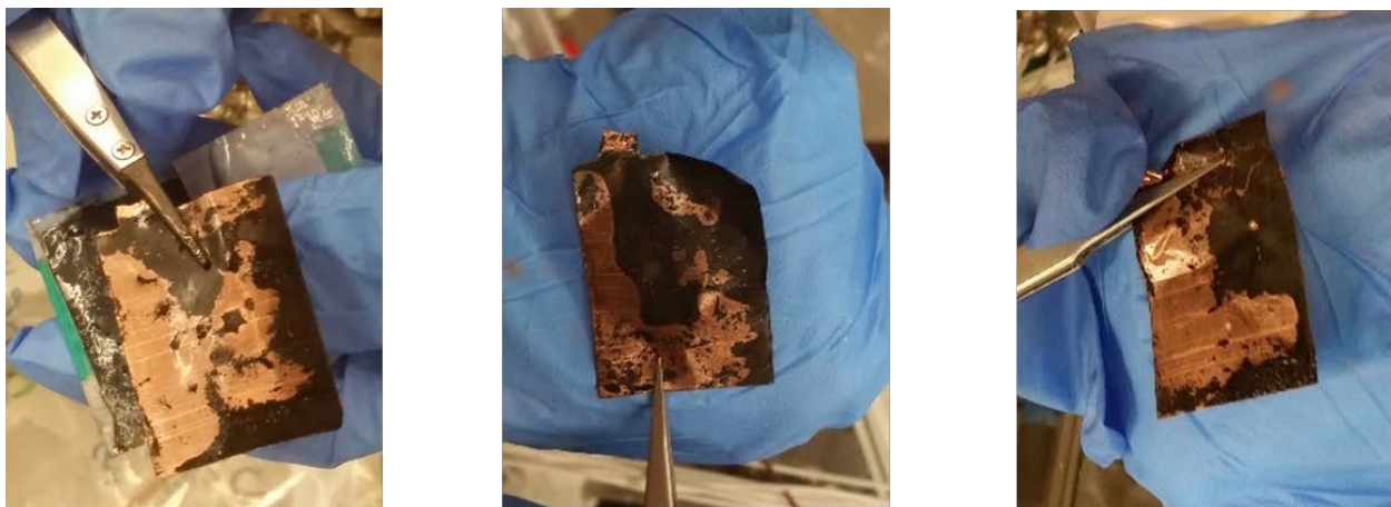
Figure 3. Harvested anode electrodes from single-layer pouch cells with baseline “GenF” electrolyte (left), “GenFM” electrolyte (center), and “GenFC” electrolyte (right) using the higher capacity-loading NMC532 cathode (A-C013B). Unexpected delamination seen on anodes, but not on cathodes. (Photos provided by Post-Test Facility).
