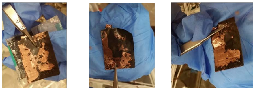
Figure 9. Opened NMC532 cells highlighting delamination problems that are associated with premature cell failure during the baseline evaluation FY19Q4 testing.
