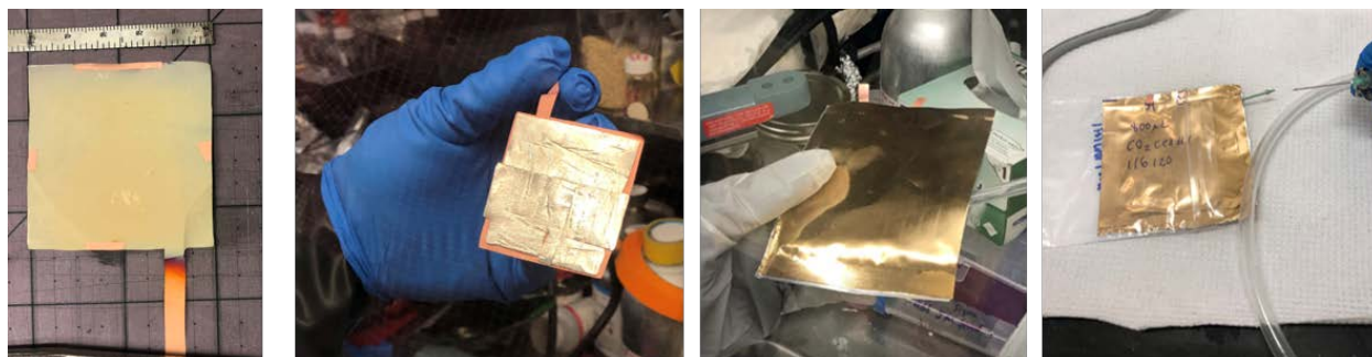
Figure 1. Images of the Si electrode (left), Li electrode (center left), pouch cell being injected with electrolyte (center right) and pouch cell injected with CO 2 (right).
