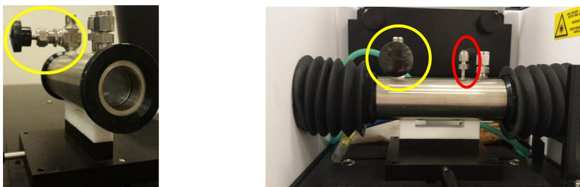
Figure 3. IR gas cell used for kinetic measurements from two different angles. The path length through the cell is 11 cm, and the KBr windows are 25 mm in diameter by 2 mm thick from Sigma Aldrich. The injection port (circled in red) is sealed with a septum, and the outgas port (yellow) can be opened for purging, if necessary.
