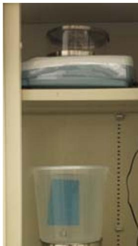
Figure 2. Buoyancy apparatus with a water bucket, indium wire to hang the pouch from the balance, and a bob (20 g dry).
